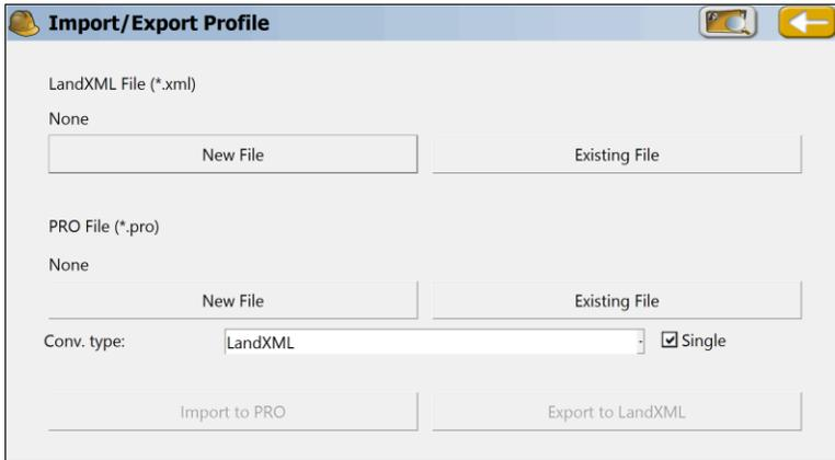
**The SurvPC Profile File Format:** It should be noted that of all the SurvPC file types that are ASCII and therefore viewable in standard text editors, the profile (.pro) file has the simplest format. The format is station, elevation, length of vertical curve, and description for road profiles. For example, the Demo.pro file that is typically provided with the software has the following four lines (which can be viewed in Notepad):
