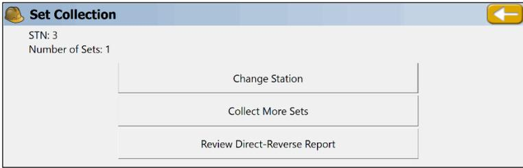
**Change Station:** This button will take you to the Instrument Setup dialog and advance the point numbers so that the original occupied point is the backsight and the last foresight point is now the occupied point.
