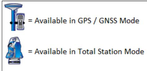
For some commands both icons will be shown, indicating that the SurvPC command can be used in both GPS and total station modes.
