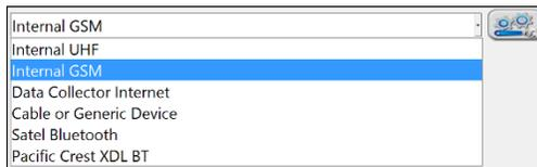
If a particular receiver model supports an internal modem or radio, meaning it is integrated into the receiver; those devices are shown first in the list. When an internal device is shown in the list, it means that model could have the device inside, but does not guarantee it. The user will have to know if the receiver was purchased with an integrated radio or modem.
