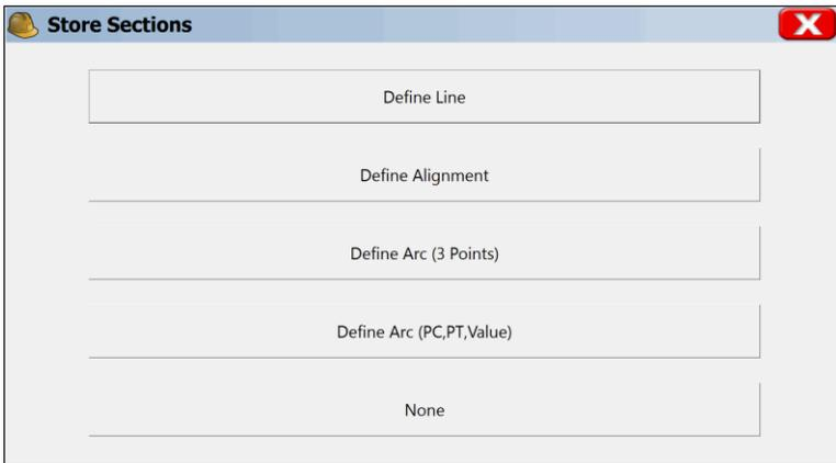
The next screen allows you to choose whether or not to store a file summarizing cross-section data. *This will be the fourth screen in the process of Define Line, Define Alignment, Define Arc (3 Point), Define Arc (PC, PT, Value).*
