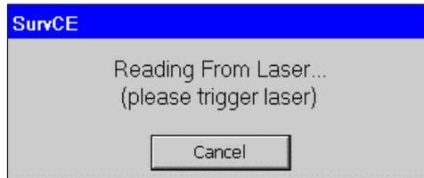
2. A progress window should pop up, indicating that Carlson SurvPC is ready to read from the laser. Aim the laser and fire at a target point. Keep firing until your laser returns a valid reading, and the progress window disappears.
