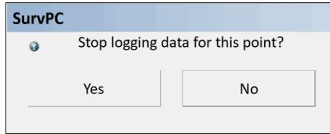
If either the Yes button in the Stop logging data for this point confirmation window or the file completes, the user will see a logging complete notification screen.
