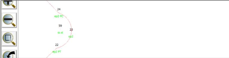
To remove the bulge in the arc and make it tangent, add code "AFIT" to point 10. If Line Details are clicked on within Configuration, the moment you add the text (click 10 directly in map screen and edit it), the line will redraw as shown below. In the field, if you add AFIT ahead of time, anticipating a bulging arc, it will draw correctly in the field.
