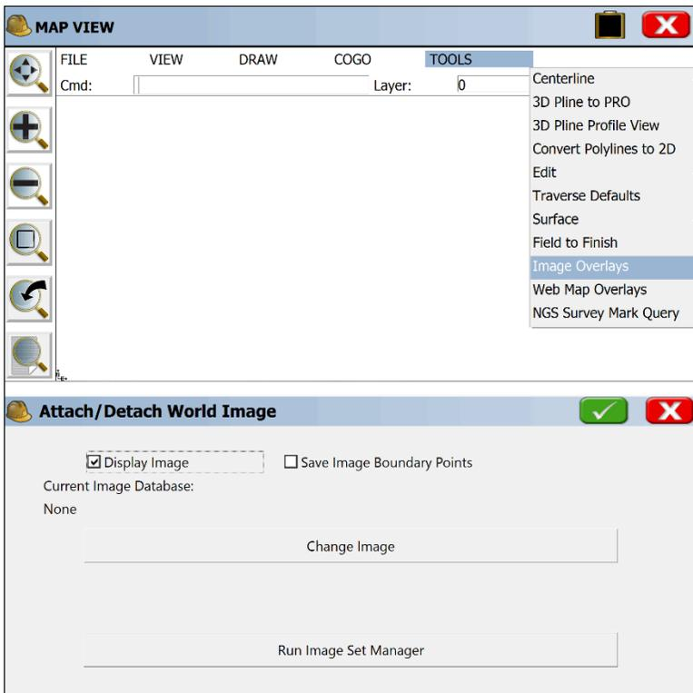
Images that do not have any georeferenced information built into them (or available in a separate jpw or tfw file) must be calibrated within Carlson X-Port, the office software companion to SurvPC, using the Image Manager. GeoPDF format is supported.
