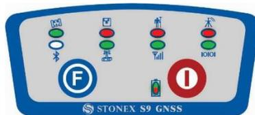
Fig. 2.17 - S9III PLUS, all led blinking at the same time
