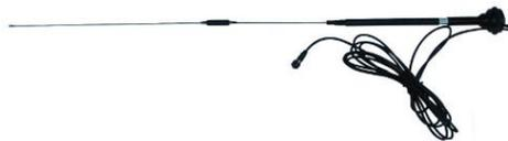
Fig. 3.9 –External radio antenna (not in scale)
