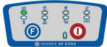
Fig. 2.8 - S9III PLUS satellite led
