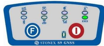
Fig 2.15 - S9III PLUS external radio led
