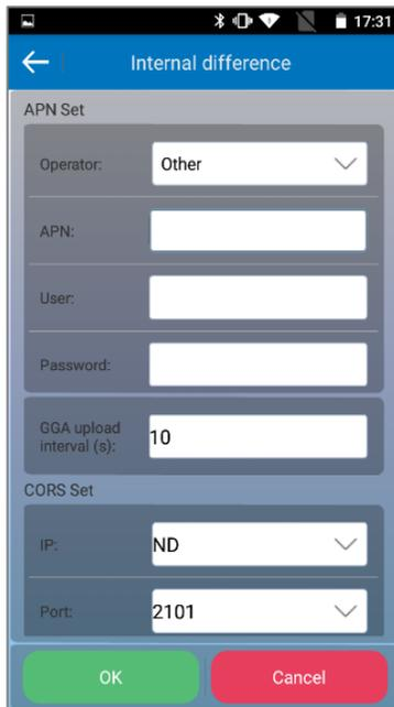
When you finish setting all internal differential parameter. Click on the "OK", and close the internal data link interface. You send the related command to set internal data link until prompts successfully. When click the button "cancel"
