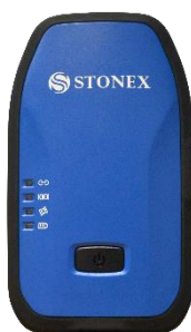
S580 Phase center L1= 121.5 mm L2= 116.5 mm
